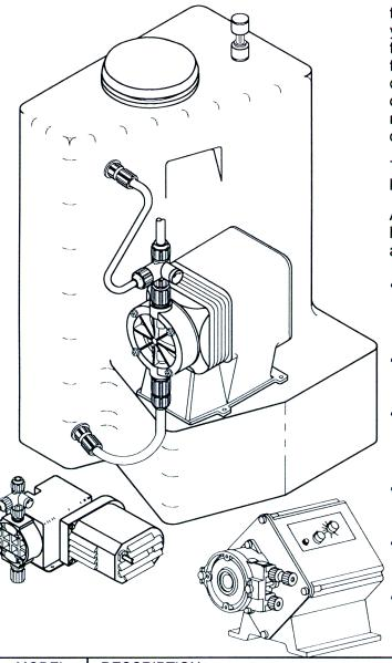
The ITS System is a completely integrated tank system constructed of high density UV resistant polyethylene (PE) with a 15 gallon capacity. This tank system is translucent with 5 gallon increments and the tank's low level indicator allows visual monitoring of chemicals without opening the tank. The tight fitting child proof lid keeps the chemical free of contaminants and protects the surrounding area from chemical fumes.
